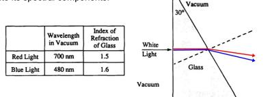
a. Determine the speed of the blue light in the glass.
